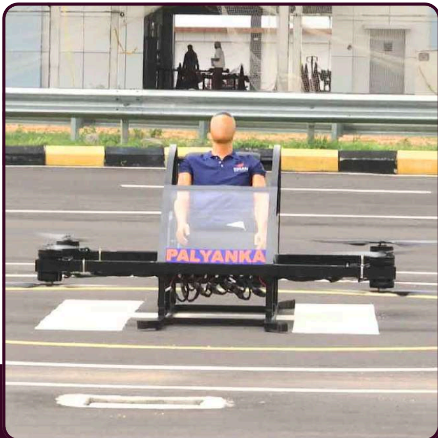
TiHAN at IITH has developed Palyanka, a heavy-payload autonomous air ambulance drone capable of carrying up to 200 kg for rapid medical evacuation, disaster rescue and cargo transport. Designed to operate without human intervention, it offers lifesaving mobility in traffic-clogged cities and difficult terrains.
